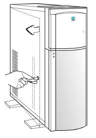
**Note:** You can not remove the key after you have unlocked the housing. You can remove it only when you lock the housing again.
